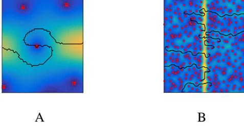
**Fig. 1.** A: an illustration of the behaviour of a contour, computed with method  $M_1$ , in the vicinity of a zero of the spectrogram; B: STFT of a noisy Dirac distribution (SNR = 0 dB) on which the first 10 contours, according to their energy content and computed with method  $M_1$ , are superimposed.
