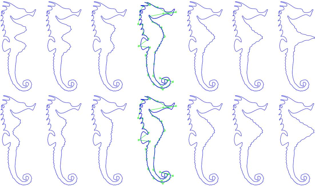
Figure 11: Multiresolution deformation of a seahorse with 512 control points. The original curve (in the middle) has been deformed by moving only one coarse control points inside and outside the abdomen. Upper row: with area preservation. Lower row: without area preservation.
