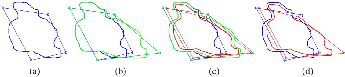
Figure 7: Shifting and loss of details. (a) original curve and coarse control polygon,  $n = 7, L = 2$ . (b) deformed curve without area constraint (green). (c) deformed curve with area constraint (red). (d) same as (c), without the green curve.
