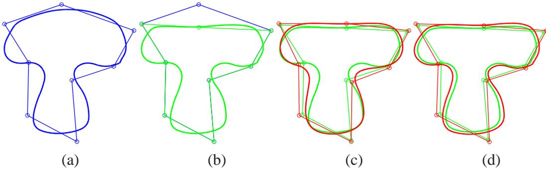
Figure 6: Influence of the coefficient  $\alpha$ . (a) original curve and its coarse control polygon (blue),  $n=5$ ,  $L=3$ . (b) deformed coarse polygon and reconstructed curve without area correction (green),  $L=3$ . (c) corrected coarse polygon and area preserving curve (red),  $\alpha = 0.5$ . (d)  $\alpha = 0.99$ .
