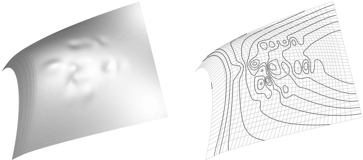
**Figure 8:** (a) Initial B-spline surface with 256 inner knot pairs. (b) Isophote analysis
