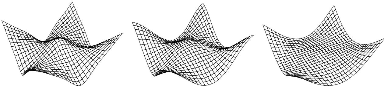
**Figure 5:** Fairing effect of the two different KRR-steps: (a) Initial surface. (b) Fairing with least-squares KRR. (c) Fairing with minimal-region KRR
