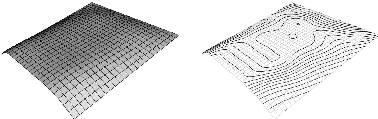
**Figure 6:** (a) Initial B-spline surface with 25 inner knot pairs. (b) Isophote analysis
