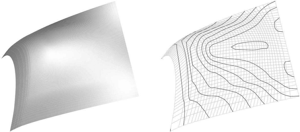
**Figure 9:** (a) The faired surface provided by the simulated annealing algorithm. (b) Isophote analysis
