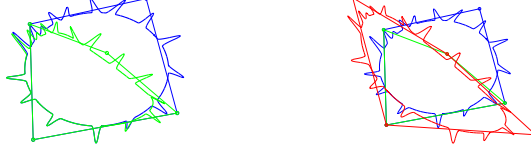
Fig. 7. Local area preserving multiresolution deformation. n = 7 , L = 2 . original curve (blue), deformed curve at level 2 (green), area preserving deformed curve at level 2 (red).
