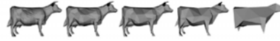
Figure 4. A sequence of approximations generated using our algorithm. The original model on the left has 5,824 faces. The approximations to the right have 194, 132, 248, and 64 faces respectively. Note that features such as horns and hooves continue to exist through easy simplification. Only at extremely low levels of detail do they begin to disappear.
