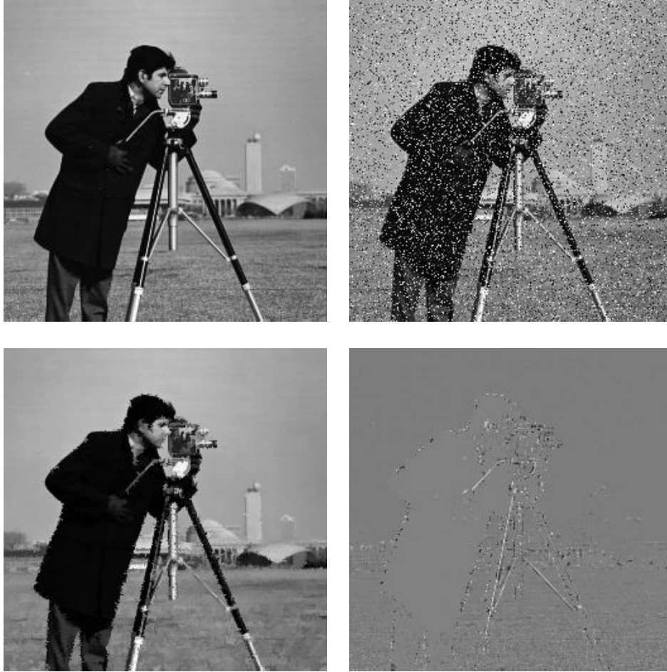
Figure 4: From left to right, top to bottom: (a) the original cameraman image u (size 256 \times 256 ); (b) degraded image v , with impulse noise intensity p = 0.2 ; (c) filtered image \tilde{v} , obtained with \varepsilon = 10^{-3} ; (d) image of the difference u - \tilde{v} . It shows that most of the noise has been removed, except at the boundaries of the objects and also in the grass texture.
